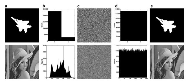
**Fig. 8.** Simulation results of LAS-IES. The top and bottom rows are the simulation procedures of binary and grayscale images, respectively: (a) plain-images; (b) histograms of (a); (c) cipher-images; (d) histograms of (c); (e) decrypted results.
