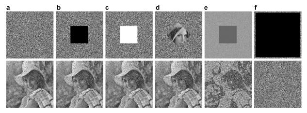
Fig. 11. Reliability analysis results of LAS-IES. The first row shows the cipher-images with noise and different kinds of data loss, and the second row shows their corresponding decrypted images: (a) 5% Saltand Pepper noise; (b) 13.56% data loss; (c) 13.56% data loss with a white square; (d) 13.56% data modification with a rotated square; (e) 13.56% data loss in the frequency domain; (f) 90.1% data loss.
