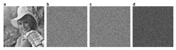
**Fig. 13.** Key sensitivity analysis in the decryption process: (a)  $D_1 = \text{Dec}(C_1, K_1)$ ; (b)  $D_2 = \text{Dec}(C_1, K_2)$ ; (c)  $D_3 = \text{Dec}(C_1, K_3)$ ; (d)  $|D_2 - D_3|$ , where  $C_1$  is the cipher-image in Fig. 12(b).
