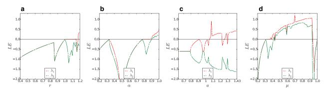
**Fig. 3.** LEs of different 2D chaotic maps: (a) 2D Logistic map; (b) 2D-SLMM with parameter  $\beta = 3$ ; (c) Hénon map with parameter b = 0.3; 2D-LASM.
