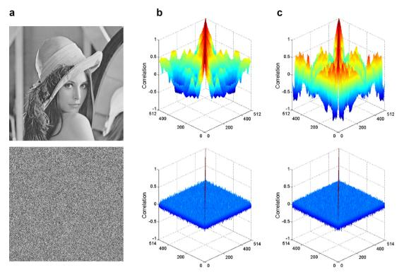
**Fig. 14.** Visualized correlation results: (a) the plain-image "Lena" and its cipher-image encrypted by LAS-IES; (b) the correlation between row pixels of (a); (c) the correlation between column pixels of (a).
